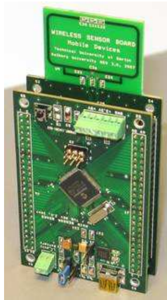
Figure 1.3: The figure is showing the second version of the mote developed by Aalborg University
