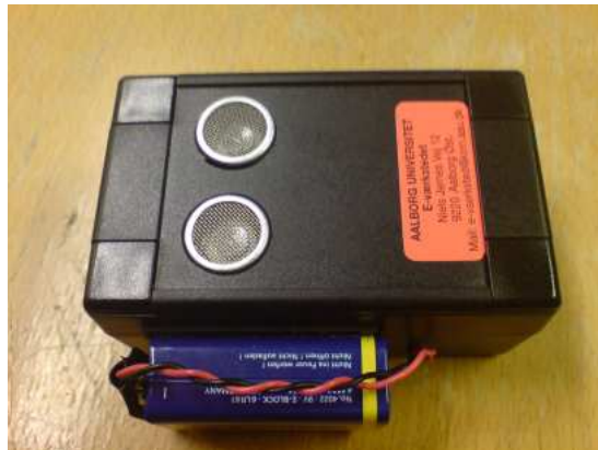
Figure 1.2: The figure is showing the distance sensor mote developed by Aalborg University
