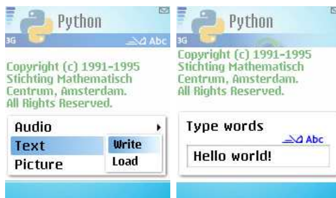
Figure 7.1: On the left figure the user selects to write a text message, on the right a message is written on the sender mobile phone
