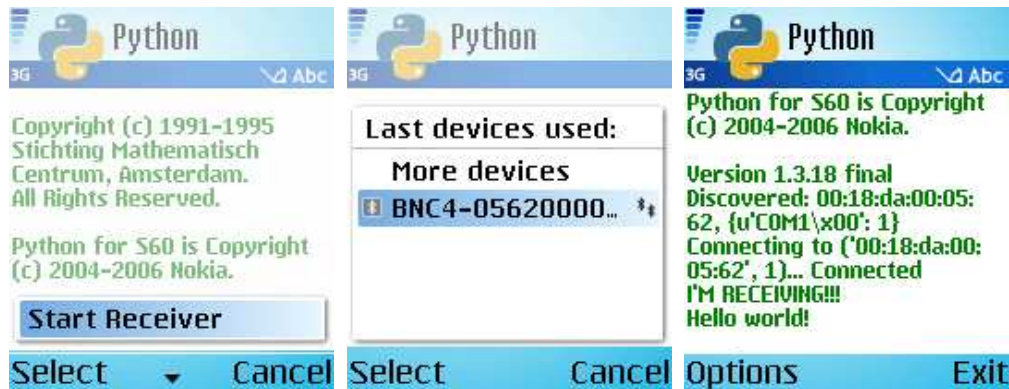
Figure 7.3: On the left figure the user is starting the receiver program, in the middle a Bluetooth search is performed and on the right the mobile phone is connected to the mote and have received the message "Hello world!"
