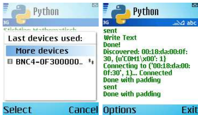
Figure 7.2: On the left figure a Bluetooth search is performed, on the right the connection is established and the message is sent into the network
