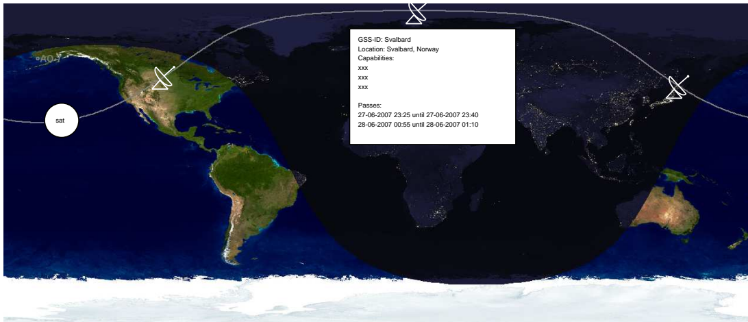
Figure 10.4: The figure shows a raw sketch of how the map presentation should be implemented. The satellite path with available passes over three different ground stations can be seen, as well as how it is possible for the satellite operator to view details of the ground stations.
